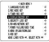
You can erase the date, time or other information from the operation display area of the playback screen. This submenu also lets you set a warning buzzer to sound for alarms or when the hard disk space reaches zero. You can set items to "OFF" as needed.
